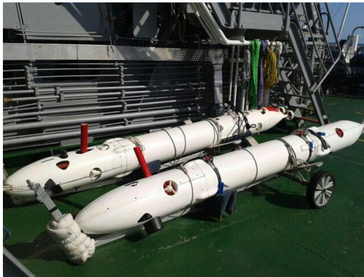
Figure 2 -The Typhoon AUVs: final versions of TifOne and TifTu on the NATO Research Vessel Alliance.
